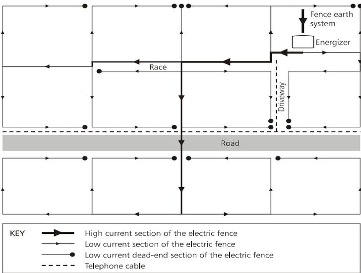
The ideal way to set up your electric fence is to feed the power out from the energizer in a 'star' fashion, with no closed loops and low currents in parts of the fence that closely parallel phone lines.
